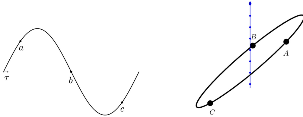
Fig. 2.1. A periodic signal (only a single period is shown) and its delay embedding in \mathbb{R}^3 with delay \tau . The points a, b, c map to A, B, C with delay coordinates.
