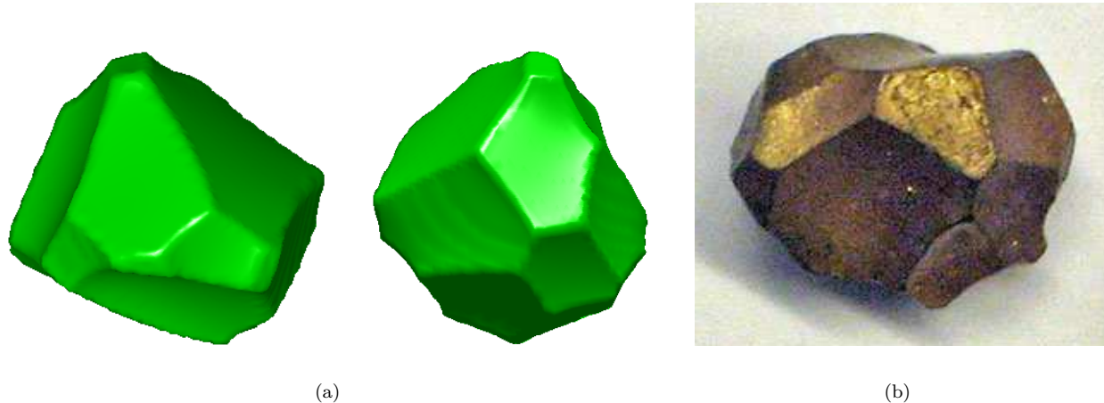
Figure 1: (a) Two views of a single grain (corresponding to a 180^\circ rotation in the xy -plane) chosen from the evolution after 300 iterations. This grain has nondimensional size \langle r \rangle = 2.11 , equal to the average grain size at this point in the evolution. The grain is very well resolved, with faces, edges, and corners all easily distinguished. (b) A single grain of beta brass, approximately 2 cm in diameter, from the collection of W.W. Mullins. The photograph is due to K. Barmak and D. Kinderlehrer. The grain compares well to the simulated grain shown in (a).
