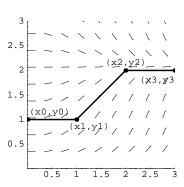
The easiest way of estimating with Euler's method is therefore to draw on the direction field the lines starting at each point and extending a distance h=1 with the correct slope, as shown. This gives  $y(1) \approx 1$ ,  $y(2) \approx 2$ , and  $y(3) \approx 2$ .
