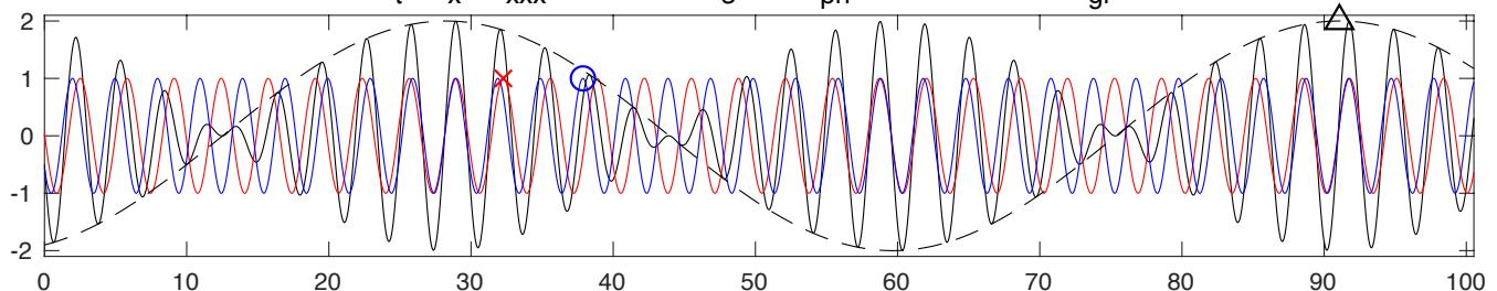
Consider ex 1 ( $\phi_t + c\phi_x = 0$ ) with general initial data  $\phi(x, 0) = f(x)$ ; the solution is  $\phi(x, t) = f(x - ct)$  (check ...); hence the solution travels at the phase velocity  $c$  without change of shape. The solution can also be expressed as a superposition of elementary waves,
