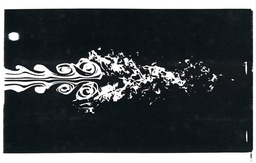
102. Instability of an axisymmetric jet. A laminar stream of air flows from a circular tube at Reynolds number 10,000 and is made visible by a smoke wire. The
