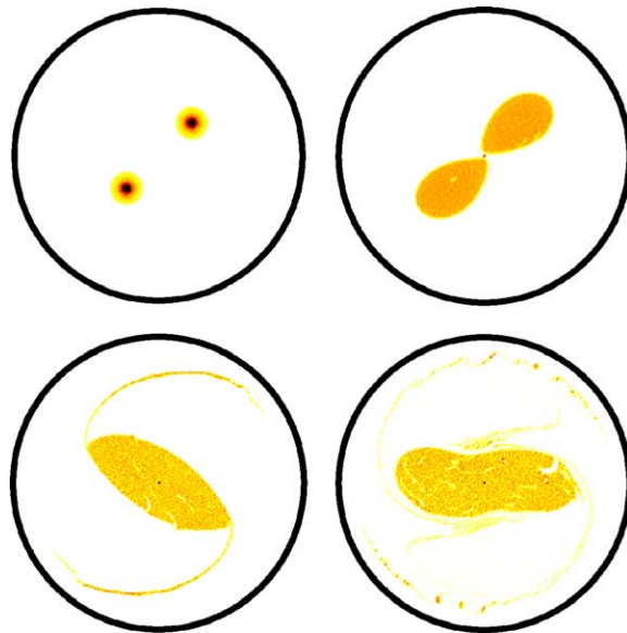
Fig. 4. Merger of two disjoint regions of electrons; time increases from left to right and top to bottom. The order of the Taylor expansion is p = 8 .
