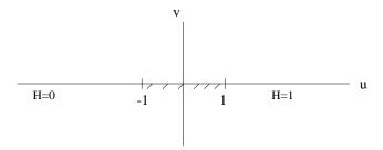
Find the steady state temperature T(x, y) in the quadrant x > 0, y > 0 when the boundary segment y > 1 on the y-axis is kept at T = 0, the temperature on the part of the x-axis with x > 1 is kept at T = 1, and the remaining boundary is insulated. The problem is indicated in the figure below.
