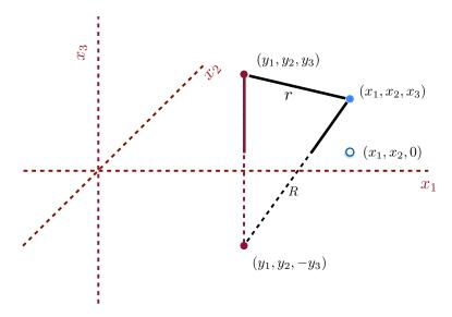
FIGURE 1. The original source location is in the upper half-space at  $(y_1, y_2, y_3)$  and the reflected image source is at  $(y_1, y_2, -y_3)$ . For target points  $(x_1, x_2, 0)$  that lie on the half-space boundary, the distances r and R from the source and image are the same, simplifying the computation of  $\mathbf{v}$  in (3.8).
